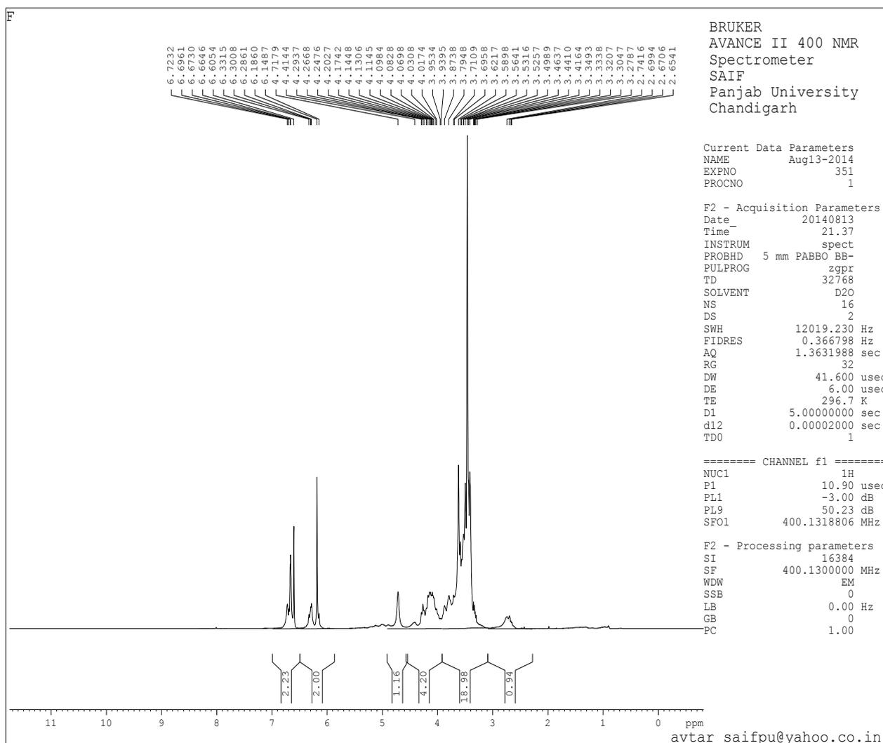
Fig. 2 :NMR spectra of Batch-1 polymer.
