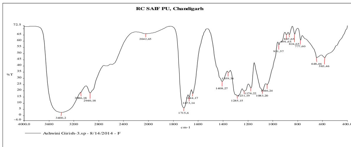
Fig.1: IR spectra of Batch-1 polymer
