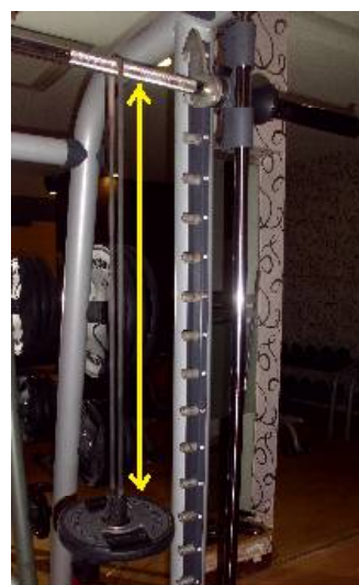
Photograph 1: The vertical portion of looped EET was measured using inch tape for understanding the magnitude of elongation under different loading conditions as compared to its length at rest.
