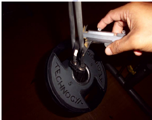
Fig. 1: Schematic side view of the experimental set up with the EET under loading with a barbell plate. A semi-circular area of EET of about 7 cm was constantly found wrapping the upper and side portions of SB but this portion was found completely flattened and thinned under loading conditions. The diameter of the supporting bar was 2.8 cm.
