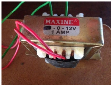
Figure 8: Step Down Transformer
