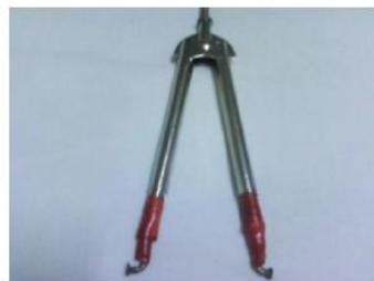
Figure3. Changed caliper for measuring distance more than 15 mm in which would be read by caliper at last.
