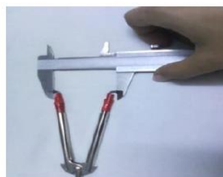
Figure 9. The distance less than 16 mm in which has been compensated by internal measure ruler
