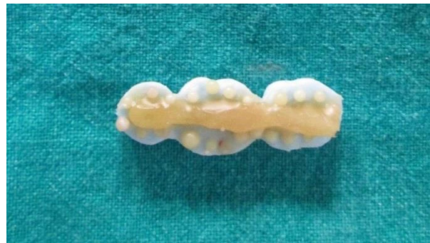
Fig 6: Wax patterns for casting.
