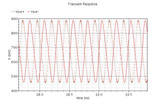
Fig. 6. The output voltage of the proposed oscillator
