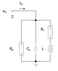
Fig. 3. The admittance looking into port 2
