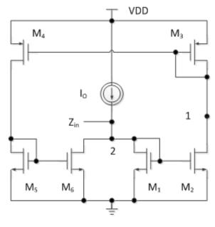
Fig. 1. Proposed current mode active inductor
