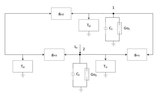
Fig. 2. equivalent network of the current mode active inductor
