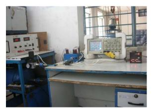
Fig. 2. Response time measuring unit
