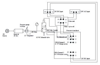
Fig. 3. Block diagram of measuring kit
