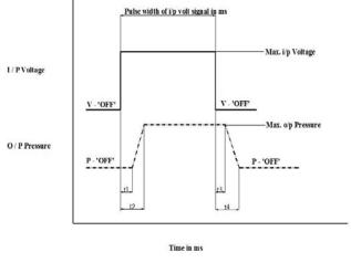
Fig. 1. Response Parameters Diagram
