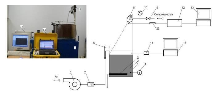
Fig. 3. Experimental stand: 1 – bath, 2 – liquid, 3 – heater, 4 – thermometer, 5 – side exhauster, 6 – fan, 7 – variable-frequency drive, 8 – blower and acoustic wave generator, 9 – valve, 10 – pressure gauge, 11 – hydrophone, 12 – data storage, 13, 15 – computer, 14 – temperature and humidity meter
