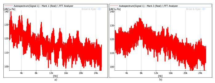
Fig. 5. Sound pressure level spectrum of acoustic wave generator when nozzle and resonator diameters ratio was equal to: a) - 1:2, b) - 1:5
