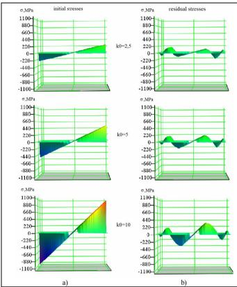
Fig. 6. Graphical stress analysis of a wire when a) entering and when b) leaving the straightener
