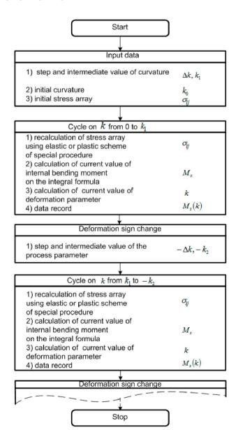
Fig. 4. Flowchart of the general algorithm for solving the problem of alternating bending.
