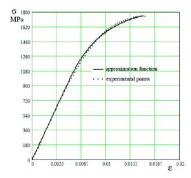
Fig. 3. Experimental stress-strain diagram and approximation function
