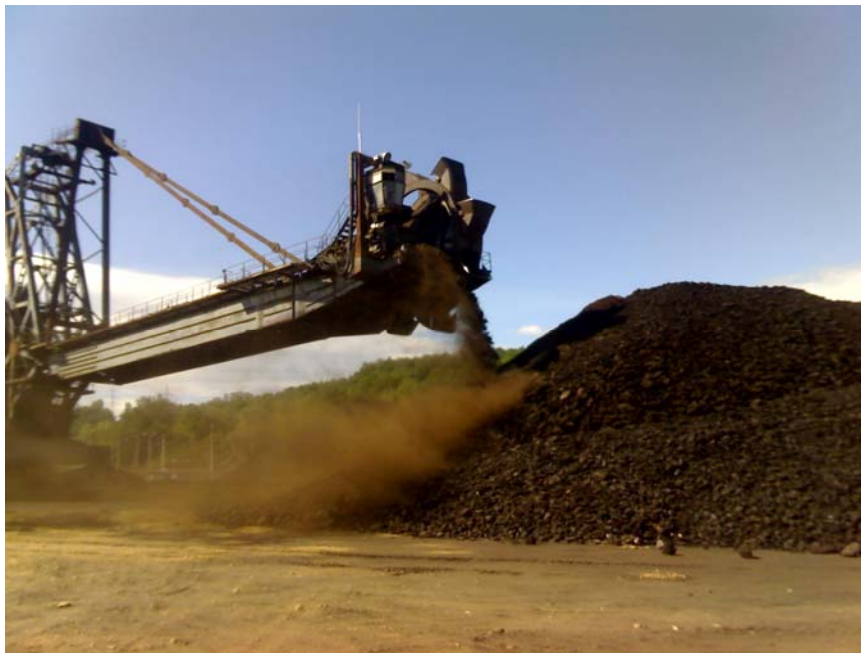
Fig.1. the depositing of coal in the deposit with the car combined of depositing/loading type KsS
