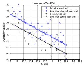
Fig.2. Log (d) versus power received in front of wood wall (blue line) and behind wood wall (red line).
