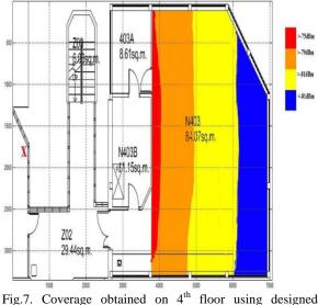
Fig.7. Coverage obtained on 4<sup>th</sup> floor using designed model.
