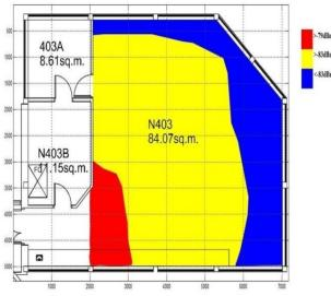
Fig.6. Signal Strength received on 4th floor.
