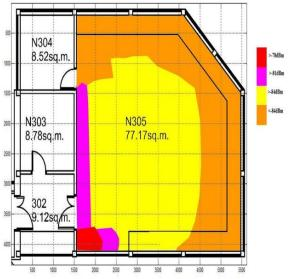
Fig.4. Signal strength received in 3rd Floor Lab.
