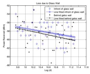
Fig.1. Log (d) versus Power Received in front and behind glass wall.
