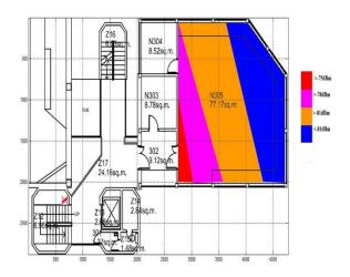
Fig.5. Coverage obtained using Designed Model.
