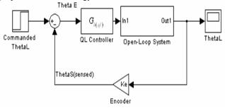
Fig.5 Closed loop feedback control diagram
