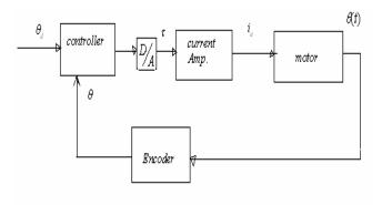
Fig.2 Block diagram of the robot joint-control system
