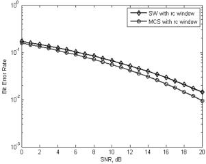
Fig.8. BER versus SNR for OFDM system with combination of MCS and windowing, and OFDM system with combination of SW and windowing.
