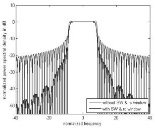
Fig.6. OFDM spectrum with SW and raised cosine window.
