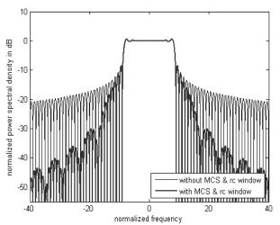
Fig.7. OFDM spectrum with MCS and raised cosine window.
