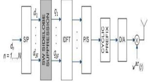
Fig.3. Block diagram of the OFDM transmitter with SW and windowing.
