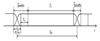
Fig.5. OFDM cyclic extension and windowing.
