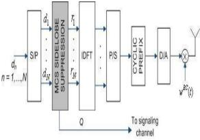
Fig.2. Block diagram of the OFDM transmitter with MCS and windowing.
