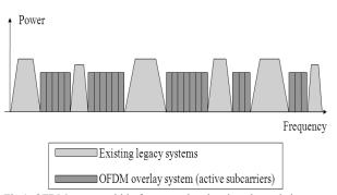
Fig.1. OFDM system within frequency band assigned to existing systems.
