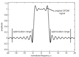
Fig.4. Block diagram of the optimization range and OFDM signal in frequency domain.
