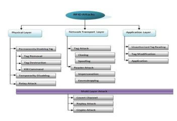
Fig.3 Classification of RFID
