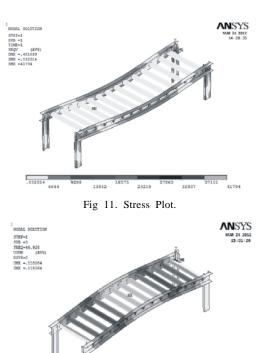
105124 .065702 001087 01314 .039421 Fig. 12. Critical Mode Shape of Optimized design.
