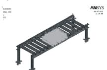
Fig. 6. A static load of 3500 N (approx 350 kg) is applied on the 4 rollers at the centre, as the deflection will be maximum, when the load is applied at the centre.
