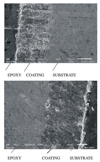
Fig. 9. Composition image of the cross-section of as-coated  $Cr_2O_3$  coating on SS-304 steel (b) on SS-310.
