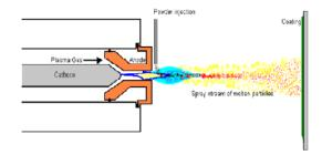
Fig. 1. Schematic Diagram of the Plasma Spray Process.
