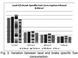
The brake Specific Fuel Consumption of the given blends depends upon the quality of combustion process. Fig. 3., shows the variation of BSFC v/s load. The reason being specific gravity of the fuel is reduced which has led to more amount of fuel to be burnt and ultimately causing the increase in BSFC value. The range of variation lies between 22 % to 4 % from 20 % blend ratio to 5 % blends No load to full load conditions respectively.
