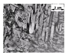
Fig. 3. Bainite Microstructure.
