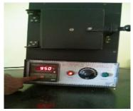
Fig. 4. Heating of Specimen in Muffle furnace.
