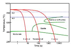
Fig. 1. Phase transformation in Austempering Process.
