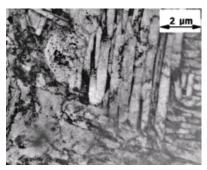
Fig. 2. Martensite Microstructure.
