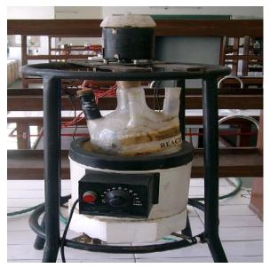
Fig. 1. Biodiesel reactor 2L capacity.
