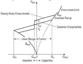
Fig. 2. The V-I characteristic of the SVC.
