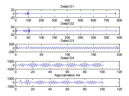
Fig. 6. DWT of voltage swell.
