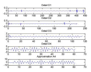
Fig. 5. DWT of voltage sag.
