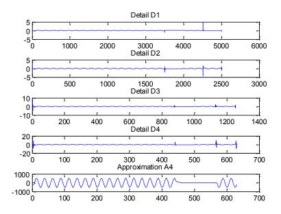
Fig. 8. DWT of voltage Interruption.
