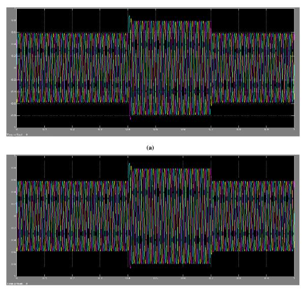
**Fig. 5.** Simulation result of an Uncompensated system. (a) voltage swell at BUS 1 (b) voltage swell at BUS 2.
