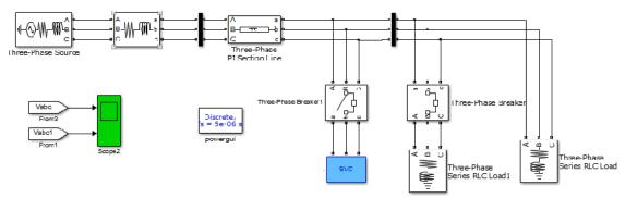
Fig. 3. SVC Compensated system for voltage sag.
