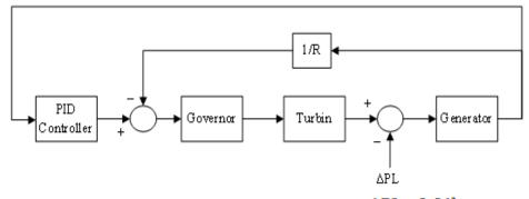
Fig. 1. A single Area Power System with the controller ( $\Delta PL = 0.01$ ).
