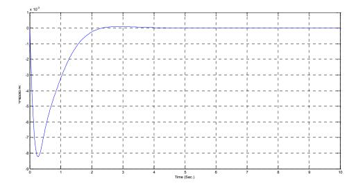
Fig. 5. Deviation of frequency of single area power system with GA based PID controller.
