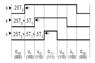
**Fig. 3.** The basic space vector and switching patterns. DC Link Current corresponding to Active Voltage Vectors.
