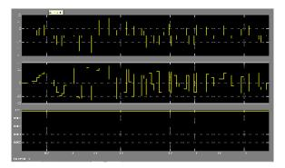
Fig.10. Three phase current measured using SCST & measurement vectors (here measurement factor is 0.01).
