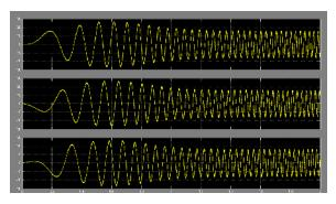
Fig. 11. Three phase current measured using SCST & measurement vectors (here measurement factor is 0.05).
