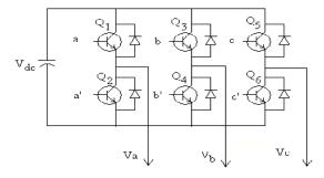
Fig. 1. Three phase voltage source inverter.
