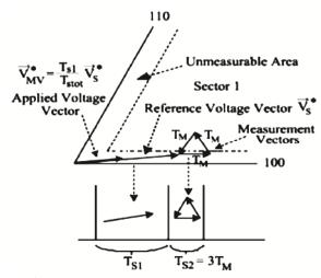
Fig. 7. Impact of measurement vectors on averaged voltage vector amplitude.
