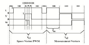
Fig. 6. PWM timing waveforms.
