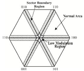
Fig. 4. Unmeasurable areas (Shaded) in the inverter output.
