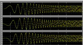
Fig. 8. Three phase current waveform measured at output terminal of voltage source inverter.
