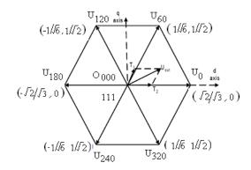
Fig. 2. The basic space vector and switching patterns.
