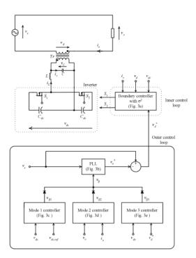
Fig. 8. Functional block diagram of the DVR [14].
