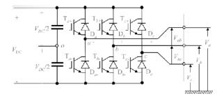
**Fig. 1.** The topology of a conventional two level VCS using IGBT switches.
