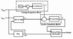
Fig. 3. Control structure for the DSTATCOM [3].
