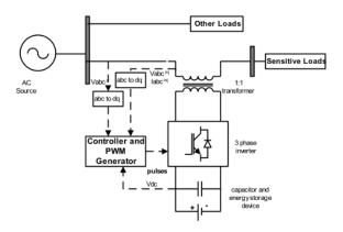
Fig. 5. Schematic diagram of DVR System.
