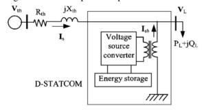
Fig. 2. Basic D-STATCOM Diagram.
