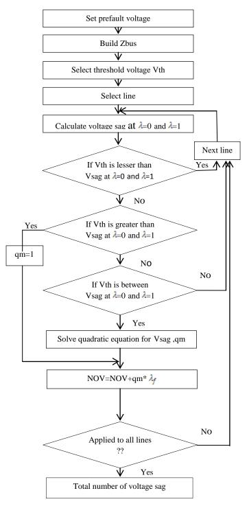
Fig 2. Flowchart for determining voltage sag and AOV.
