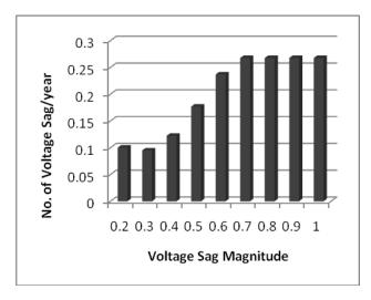
Fig. 5. Number of Voltage sag at bus 8.
