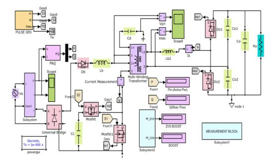
Fig. 7: Simulink model Developed for proposed converter.
