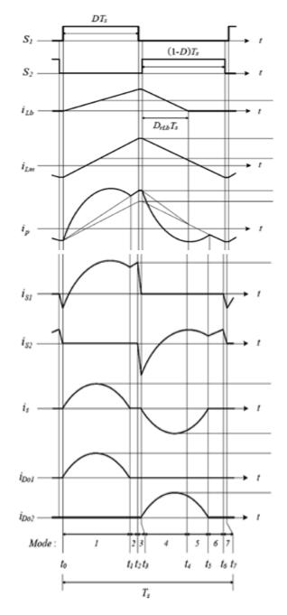
Fig. 6. Key waveforms of the proposed converter.
