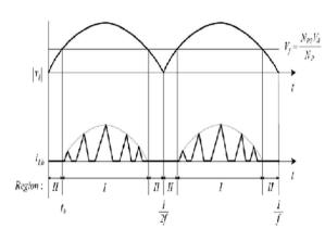
Fig. 5. Operation region of Converter.
