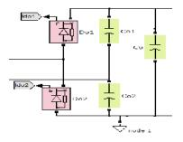
Fig. 4. Voltage doubler rectifier schematic.
