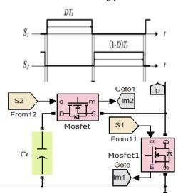
Fig. 2. Active clamp circuitry.
