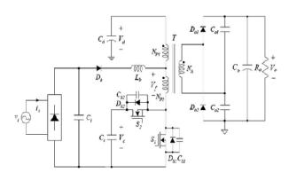
Fig. 1. Circuit diagram of proposed single stage soft switching converter.
