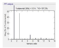
Fig. 9. FFT Analysis of Supply Current.
