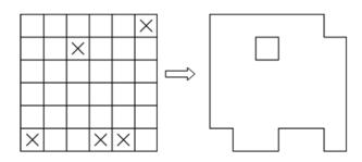
Fig. 1. Microstrip patch to be optimized.
