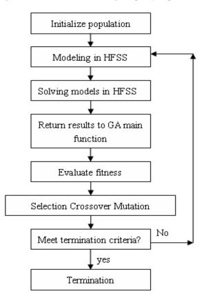
Fig. 2 Flowchart representing HGA apply to micro strip patch.
