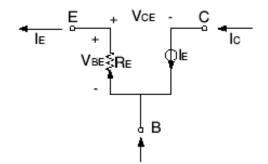
Fig. 2(a). Equivalent circuit model of fig 2.
