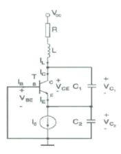
Fig. 2. Schematic of the Colpitts oscillator.
