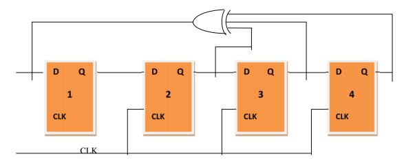
Fig. 3. Logic Diagram of Pseudo Random Binary Sequence Generator.
