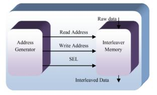
Fig. 2. Top level View of WIMAX Interleaver.
