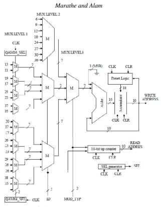
Fig. 1. WiMAX Address generator.
