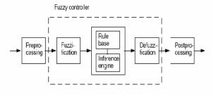
Fig. 3. Structure of fuzzy logic controller.
