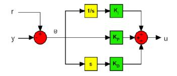
Fig. 2. Traditional PID structure.
