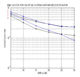
In Fig. symbol error rate at 0.106 is taken and different values of the Signal to noise ratios are seen for different type of estimators *i.e.* MMSE or LS and the modified versions of these estimators with tap of 10 is used. So they are called as MMSE10 and LS10 estimators and the results are shown in Table 1.
