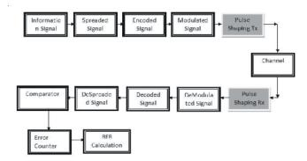
Fig. 1. Block diagram for WCDMA System.
