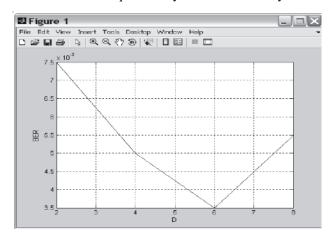
Fig. 14. BER versus Group delay D for WCDMA at 5MHz.
