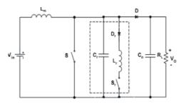
Fig. 2. Circuit diagram of the soft switching of boost converter. Fig. 2 shows the proposed Snubber topology for the boost
