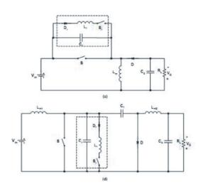
Fig. 4. Four basic circuits of DC/DC converters with soft switching.
