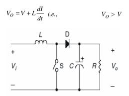
Fig. 1. Basic boost converter.
