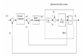
Fig. 7. Simplified block diagram of an induction servomotor drive.
