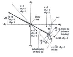
Fig. 6. Sliding line control in phase plane  $X_1 - X_2$ .
