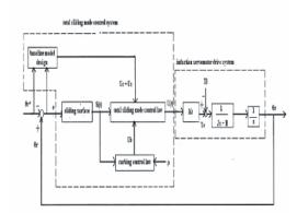
Fig. 8. Block diagram of Total Sliding Mode Control system.
