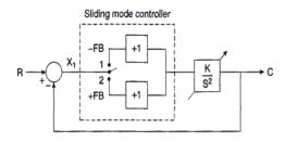
Fig. 3. Variable structure control of second order system.
