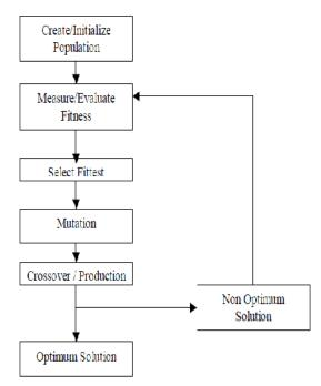
Fig. 4. Genetic algorithm process flowchart.
