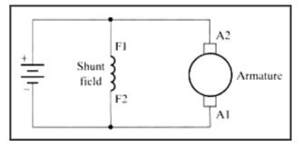
Fig. 1. DC shunt Motor.
