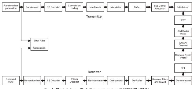
Fig. 1. Physical Layer Block Diagram based on IEEE802.22 WRAN.
