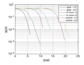
Fig. 3. Coded BER curve for different modulation at different code rates over AWGN channel.
