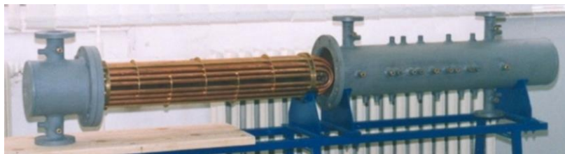
Fig. 1 Laboratory STHE with cross segmental baffles
