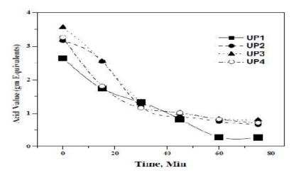
Fig 1: Acid value of all unsaturated acid UP1, UP2, UP3 and UP4 at different time intervals.
