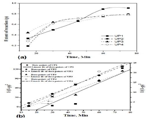
Fig 2: Plots of (a) extent of reaction of different unsaturated polyesters with time and (b) Average degree of polymerization of different unsaturated polyester with time.
