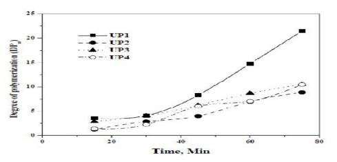
Figure 3: Degree of polymerization of different unsaturated polyesters with time.
