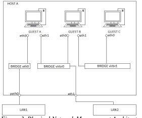
Figure 3. Physical Network Management Architecture
