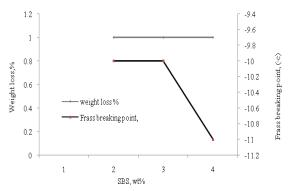
Fig 4: The effect of SBS wt% variations on the Frass breaking point and weight loss (2 wt% bentonite)
