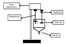
**Fig 1:** High-speed and high shear double –mixer set *Penetration Index (PI) Estimation*
