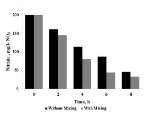
Fig. 6: Effects of reactor mixing on nitrate reduction rate in BER (Initial NO<sub>3</sub>=200 mg L<sup>-1</sup> NO<sub>3</sub>, Current density=8 mA/cm<sup>2</sup>)
