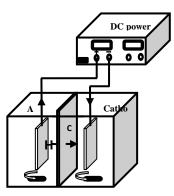
Fig. 1: Schematic diagram of the bioelecterochmical reactor
