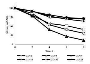
Fig. 5: Simultaneous effects of current density and running time on nitrate reduction
