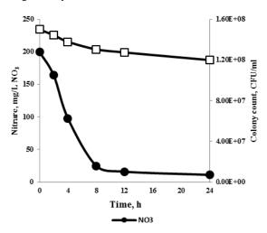
Fig. 4: Influence of running time on nitrate reduction rate and viability of denitrifying bacteria in BER (Initial NO3 =200 mg L<sup>-1</sup> NO<sub>3</sub>, Initial bacteria=  $3 \times 10^{8}$ , Current density= $8 \text{ mA/cm}^2$ )
