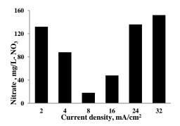
**Fig. 2:** Effect of current density on bioelectrochemical nitrate reduction (NO<sub>3</sub><sup>-</sup>=200 mg L<sup>-1</sup> NO<sub>3</sub><sup>-</sup>, Time=8h)
