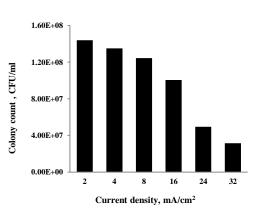
**Fig.3:** Effect of current density on colony count of denitrifying bacteria in BER(NO<sub>3</sub>=200 mg  $L^{-1}$  NO<sub>3</sub><sup>-</sup>, Time=8h)
