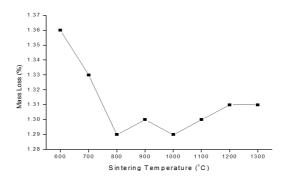
Figure 3: Percentage of Mass Loss of BNT Ceramic with x=0.15 at Different Sintering Temperature
