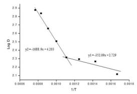
**Figure 5: Activation Energies of Grain Growth**
