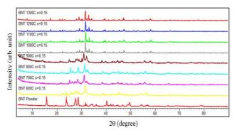
Figure 1: XRD Pattern of BNT Ceramic with x=0.15 for All Sintering Temperatures
