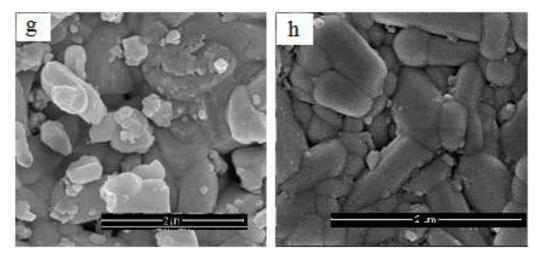
Figure 4: Microstructure of BNT Ceramic for All Sintering Temperatures; (a) 600°C, (b) 700°C, (c) 800°C, (d) 900°C, (e) 1000°C, (f) 1100°C, (g) 1200°C, and (h) 1300°C
