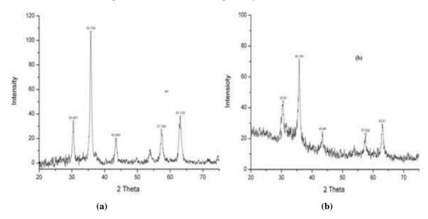
Figure 1: XRD Patterns of Olive (a) and Flaxseed (b) Oils Mediated SPIONs
