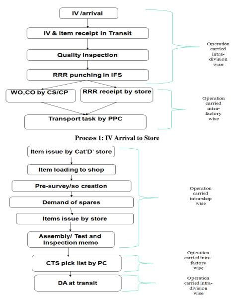
Process 2: Issue to Instrument Shop to Repair and Overhaul Completion, Testing and Dispatch Figure 1: Process Mapping of Repair and Overhaul Process
