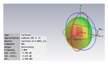
Figure 3: Radiation Pattern of RMPA Showing 76.29% Total Efficiency & 6.393 dBi Directivity
