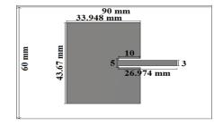
Figure 1: Dimensional View of RMPA at 2.058 GHZ (All Dimensions in mm)
