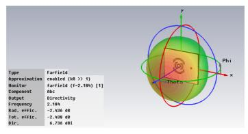
Figure 6: Radiation Pattern of the RMPA along with the Suggested Material Cover Showing Total Efficiency of 75.62% and the Directivity 6.736dBi
