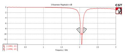
Figure 2: Simulated Result of RMPA Showing Return Loss of -14 dB and BW of 36.6 MHz
