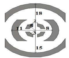
Figure 4: Dimensional View of the Suggested Cover (All Dimensions in mm)
