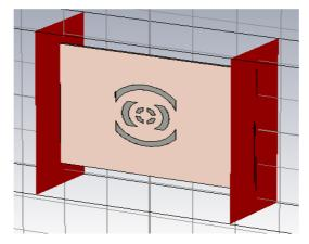
Figure 7: Suggested Material Cover Placed between the Two Waveguide Ports
