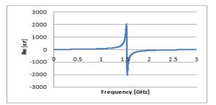
Figure 8: Permittivity versus Frequency Graph
