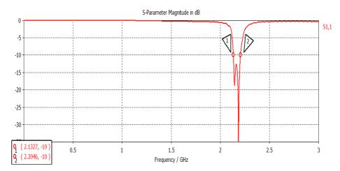
Figure 5: Simulated Result of the RMPA along with Suggested Material Cover Showing Return Loss of -35 dB and Bandwidth of 71.9 MHz
