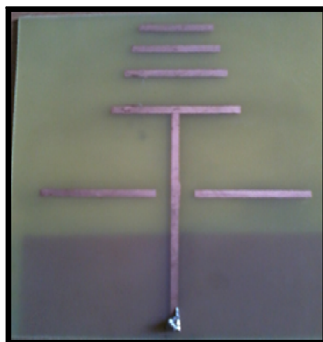
Figure 3: The Fabricated Layout of Proposed Microstrip Yagi-Uda Antenna
