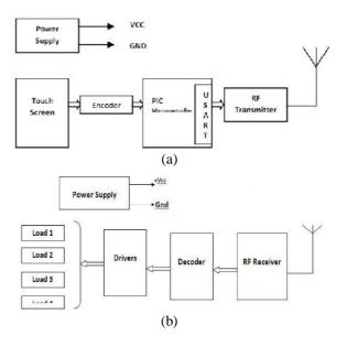
Fig.1 Functional Block diagram of proposed system (a) Transmitter Module and (b) Receiver Module
