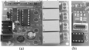
Fig. 4 RF Modules (a) Transmitter (b) Receiver
