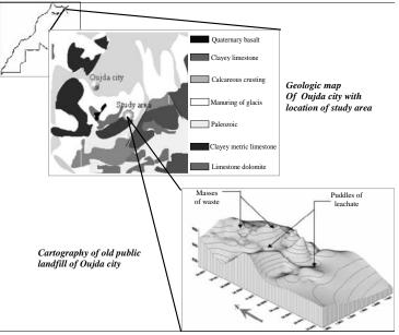
Figure 1: Geological map of the landfill's setting
