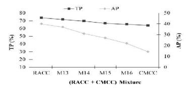
**Figure 5:** Variation in total porosity and aeration porosity of substrates resulting from mixtures of Raw Acacia cyanophylla compost (RACC) with cattle manures Co-compost (CMCC)
